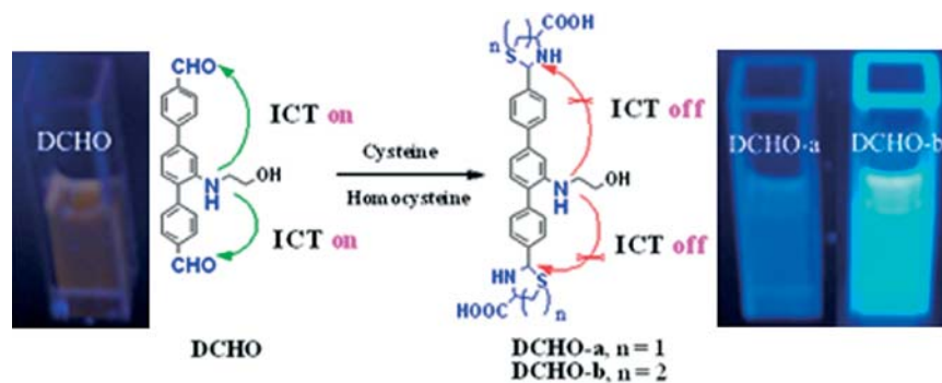
Scheme 3. Reaction of DCHO with Cys or Hcy to afford thiazolidine ( DCHO-a ) or thiazinane ( DCHO-b ) and the change in fluorescent colour on excitation at 365 nm using UV light at room temperature.
